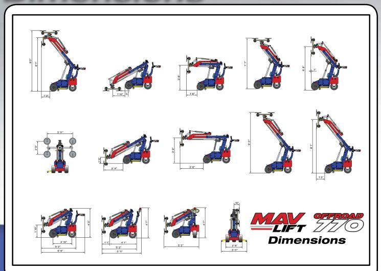
Couple the range of the Advanced Articulating Joint and the MAVLift's signature Synchronous Controls, (which ensure a constant inclination angle of the vacuum unit) and you have a high performance and versatile lifting robot.
