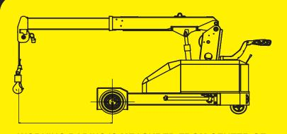
WORKING RADIUS IS MEASURED FROM CENTER OF FRONT WHEELS TO THE CENTER OF SUSPENDED LOAD
